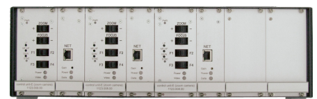
6-camera rack equipped with three camera modules and three video servers
