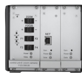
Single-camera rack with video server
