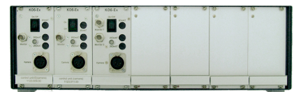
6-camera rack with camera control modules
