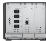
Single-camera rack with video server
