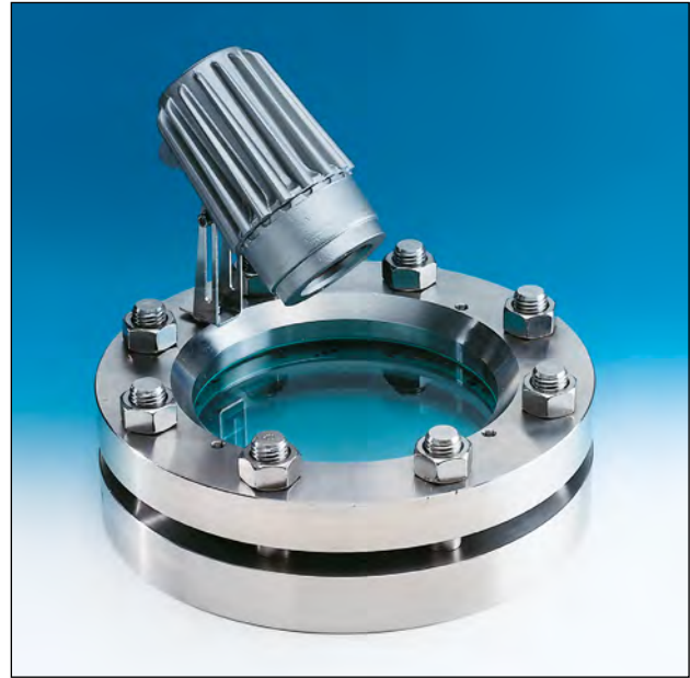
Lumistar luminaire USL 05 application as combined sight and light port on a sight glass fitting acc. to DIN 28120, mounting by way of hinged bracket
