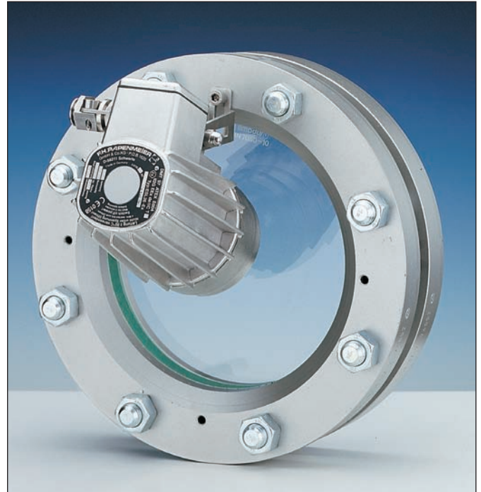
Application as a combination of sight and light glass mounted onto a circular sight glass fitting DIN 28120 (with hinged bracket)
